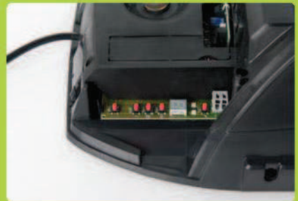
Multi-segment display for programming and status indication
